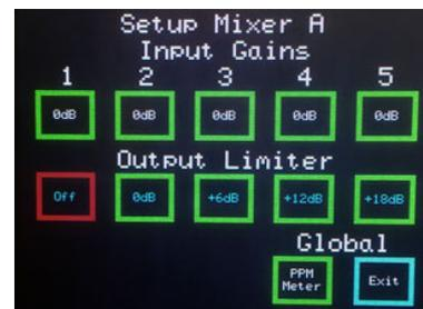
The Mixer output limiter can be switched out of circuit (off) or selected to limit at 0dBu, +6dBu, +12dBu or +18dBu. Just touch the required preset, again the selected button will turn red.
